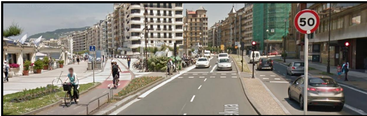
San Sabastian street scene with segregated cycle paths and shared space paths. Paths are continuous and use one of two designs throughout depending on street type.
